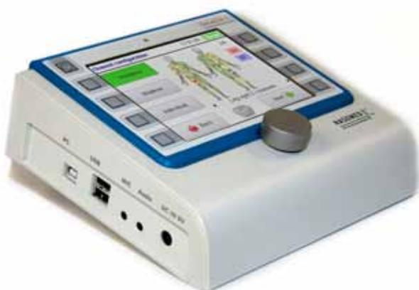
Apart from the modified appearance, the new stimulator RehaStim2 offers an even simpler operation. Via a rotary knob, the existing eight stimulation channels are assigned and defined with corresponding parameters.
